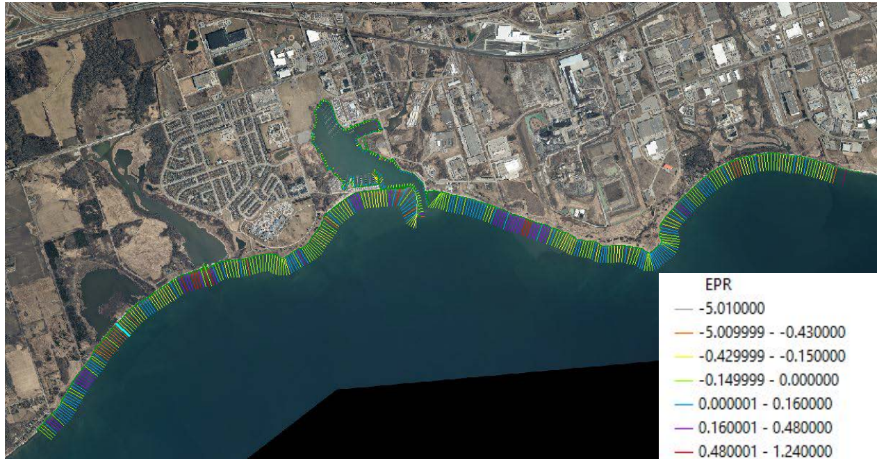
Figure 14: Rate of shoreline change (EPR m/year) along the shore from 2005-2018 (all negative signs show erosion, whereas the positive shows accretion)
