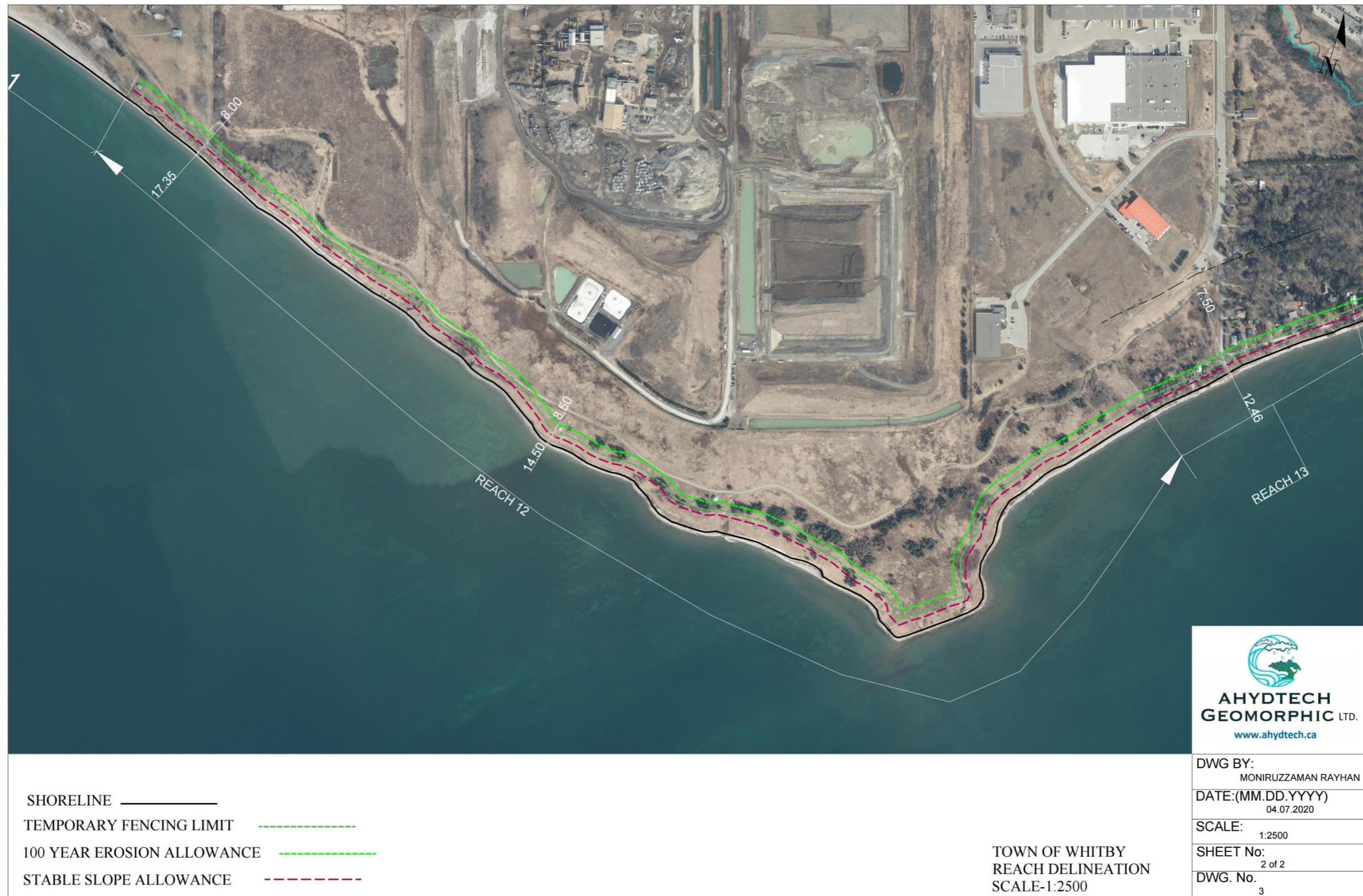
Figure 37: Erosion hazard limit at Reach 12.
